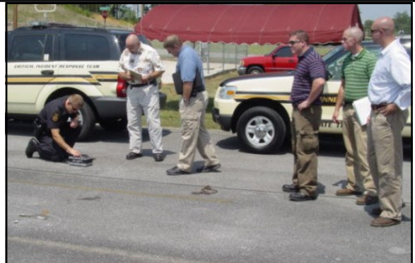
The drag factor of the road was measured using a drag sled and accelerometer.
